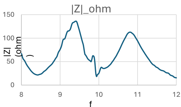
Figure 9: Complex impedance, |Z| as a function of frequency for \text{Ba}_2\text{CoZnFe}_{12}\text{O}_{22} .
